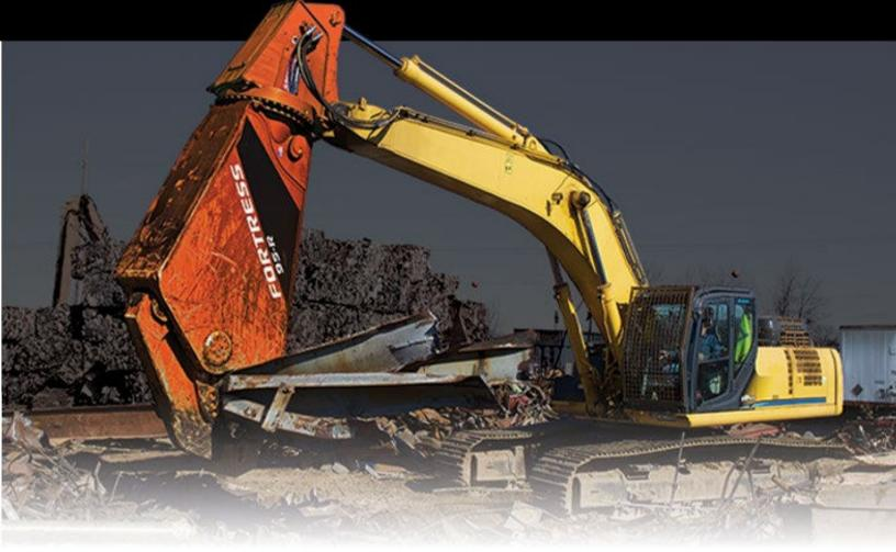
Fortress mobile shears can be installed on a variety of carriers; everything from smaller excavators up to massive high reach machines. All shears are rated for up to 5500 psi.
