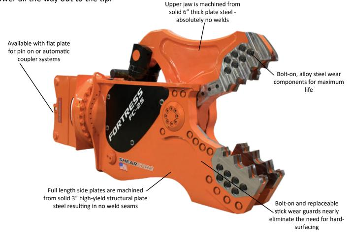
Why call it a Demolition Shear? The Fortress FC is a new class of tool with unique construction and capabilities. It utilizes a solid upper with no welds and press-fit pivot group (like our shears) allowing for tolerances tight enough to shear rebar all the way out to the tip.
