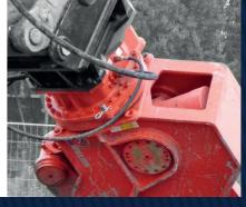
The speed valve developed by Rotar allows the jaws to close quickly and automatically switch from speed to power mode as soon as the job requires
