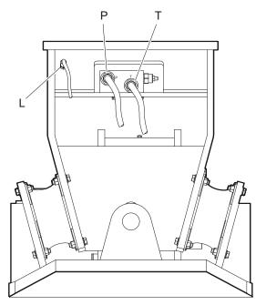
Connect the leakage oil hose to port »L«, making sure it is torsion-free.
