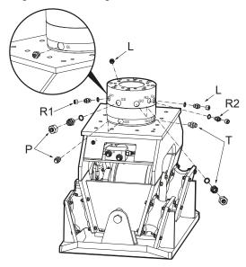
Install the hoses at the connections »P«, »T« and »L« as shown below.
