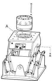
Align the rotating mechanism according to the markings to make sure the screws can slide through the rotation mechanism into the holes in the outer housing.
